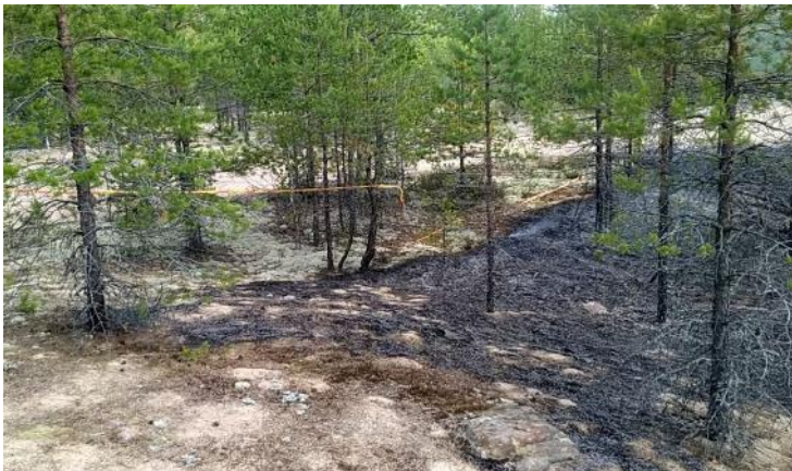
The spread of the fire stops at the edge of the area where the ForExt water mixture has been applied.
