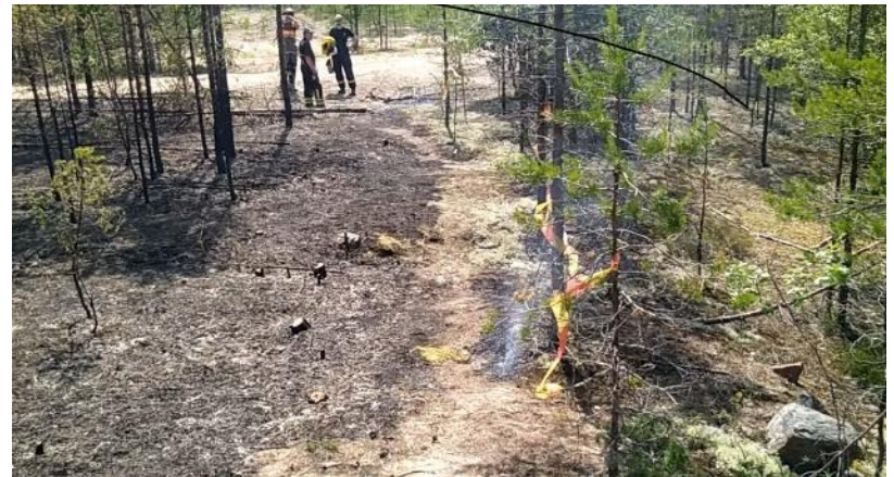
The spread of the fire stops at the edge of the area where the ForExt water mixture has been applied.
